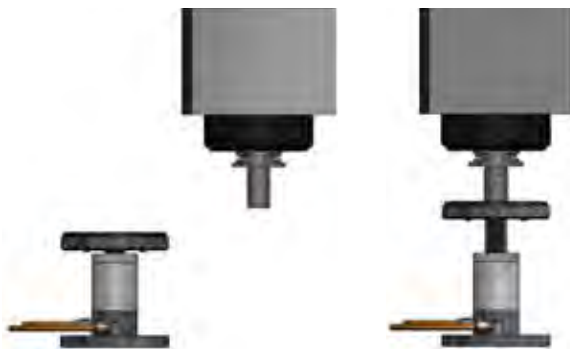
Locating of the cup using the machine's spindle and the special locator tool
