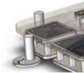
Pin-Stop during workpiece positioning
